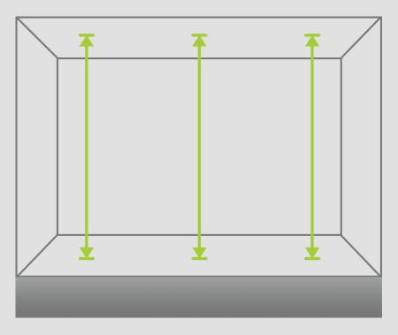
Measure the total floor to ceiling height at (recommended) 650mm from the back wall at the three points indicated in the diagram, make a note of the SMALLEST of the three measurements. This will be the measurement we will use to manufacture your sliding wardrobe. Do not deduct any measurements for liners, tracks, etc, these will all be taken into consideration, prior to manufacturing. We do all the maths so you don't have to.
